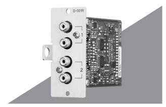
The D-001R is a line input plug-in module designed for use with the M-9000. It has 2-channel unbalanced input of RCA jacks. Input signals to both channels are mixed together. The D-001R can process effect for TONE/EQ/COMPRESSOR to two inputs independently.
