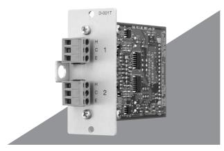
The D-001T is a plug-in module designed for use with the M-9000 and can provide two independent balanced inputs. The D-001T can handle signals ranging from microphone level to line level by controlling their input sensitivity in 9 increments from -60dB to -10dB.
