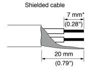
Expose 8 mm (0.31") or more when using the above ferrule terminal, and cut off an extra conductor protruding from the sleeve.
