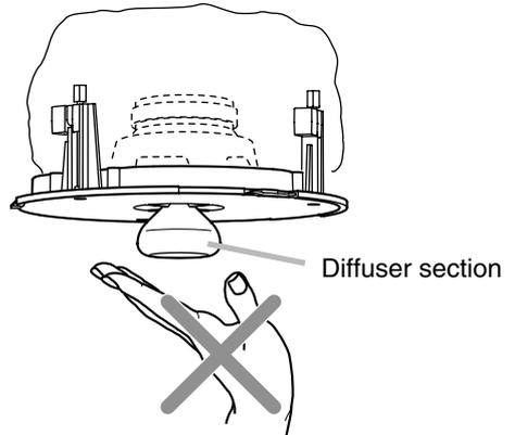
Rotate and tighten the mounting tab axis screws (3 places) on the unit clockwise to their full stop in order to grip the ceiling panel with the mounting tabs.
