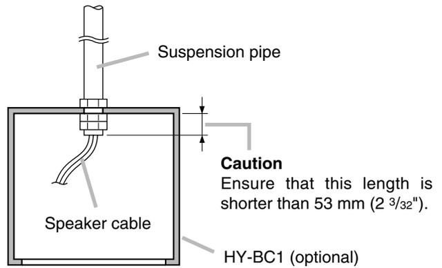
**Step 3. Connect the speaker cable to the push-in terminal.**
