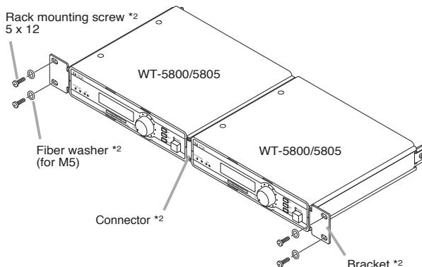
\*2 Component parts of the MB-WT4.
