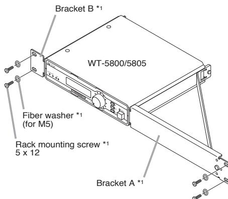
\*1 Component parts of the MB-WT3.
