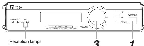
**Step 1.** Turn the power on, and the LCD screen comes to display the receiving frequency and RF/AF levels.
